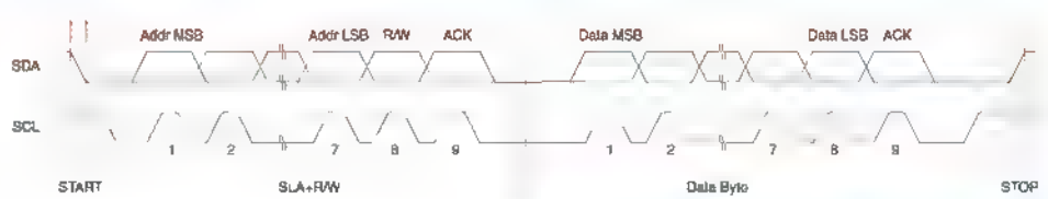
Figure 1: Typical I 2 C timing diagram.
